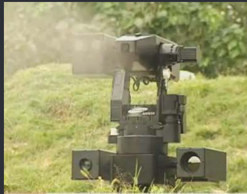
Sentry used to guard the Korean DMZ, fires autonomously
